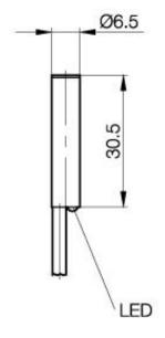
Inductive Sensors BES 516-372-E4-C-PU-03 D6.5 x 30.5 normally-open Sn=1,5mm shielded
